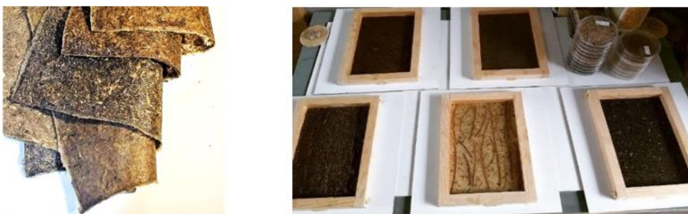
Image 8: Vinyl of gelatin and starch bioplastic with fibre. The optimal formula for the matrix was 10:3/4:2:1, which entails 100 g water, 7.5 g of gelatin, 20 g of glycerin and 10 g of vinegar for the mould used. The optimal amount of fibre added was 3 g dried or 20 g wet. It solidifies in 15 minutes, but to be completely dry takes approximately 96 hours.
