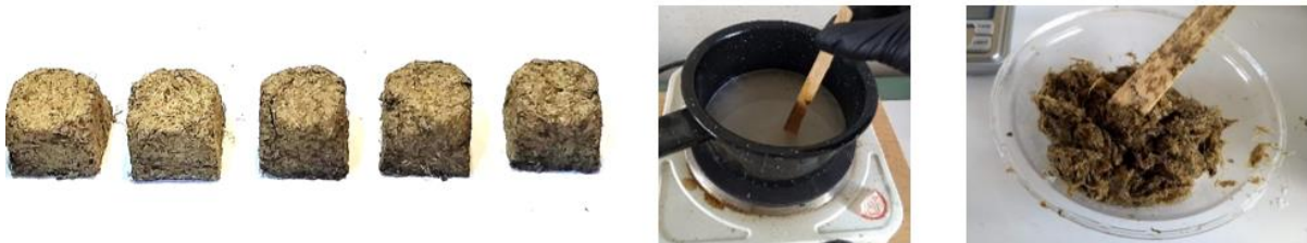
Image 7: Agglomerate with starch bioplastic. The optimal matrix was composed by a 4:1:1:1: 1/5 formula: water 30 g, starch 7.5 g, vinegar 7.5 g, glycerin 7.5 g, with 1.5 g of dried fibre. The difference between this material and the previous one is that this were not subjected to pressure to give form. It was just cast into the mould and left to dry. It takes around 4 days to be completely dry.
