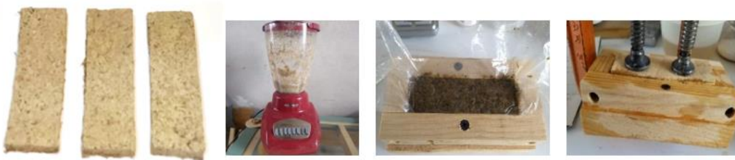
Image 5: Paper. A laminate from a mixture of 80% water hyacinth fibre and 20% recycled newspaper, both previously treated with water immersion of 7 days to soften the fibre.
