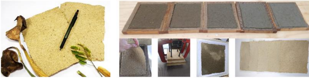
Image 5: Paper. A laminate from a mixture of 80% water hyacinth fibre and 20% recycled newspaper, both previously treated with water immersion of 7 days to soften the fibre.
