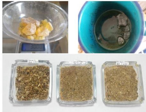
Image 9: Bioplastic of pine resin. This material consists of three components: pine resin, beeswax and fibre. The wax is added to give fluency to the mixture. The optimal amount was 15 g resin, 15 g wax and 3 g dried fibre. The matrix is heated until it melts and then is cast in a mould with the fibre already inside it, stirred for a few seconds and left to dry.
