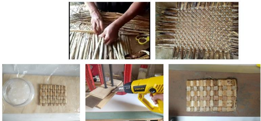
Image 10: Bio-laminated weave. This material consists of a piece of woven stems and a process of bio-laminate with starch bioplastic. First, the hyacinth stems are set in the sunlight for drying, then the air is removed by pressure with the hand. Once the stems are flat, the weaving starts. The bio-laminated weave consists of mechanical pressure applied to the piece of woven stems. Once it is flat, it is coated with layers of starch bioplastic, then is subjected to pressure again, with a source of heat supplying hot air to dry and harden the piece.
